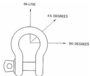
Side loads should be avoided as the products are not designed for this purpose. If side loads cannot be avoided, the following reduction factors must be taken into account:
