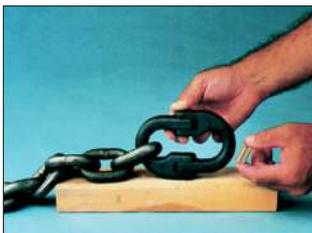
1. Place the locking sleeve between the assembled half link forgings.
