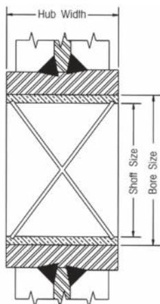
Roller Bearings are designed to operate on shafts carburized to 60 Rockwell C and grounded to +/- .0005 of shaft size.
