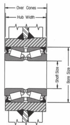
Tapered Bearings are designed to operate on shafts machined to +/- .0005 of shaft size. Applications should provide for tightening separator plates against bearing cones to adjust and insure proper function of bearings.
