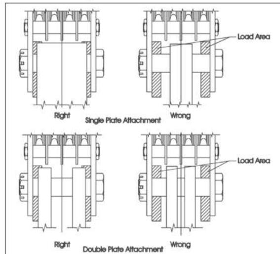
NOTE: The outside of attaching plates must be within the indicated load areas. Means must be provided to keep attaching plates equally spaced from the block side plates. For dimension information, including the load area, visit [www.mckissick.com](#).
