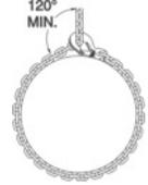
In shortening applications, a 20% reduction of the Working Load Limit is required except when using the Crosby A-1338 Cradle Grab Hooks, S-1311 Chain Shortener Link, the A-1355 Chain Choker Hook in conjunction with the S-1325 Chain Coupler Link, or the Crosby Eliminator® shortener link. They can be used without any reduction to the Working Load Limit.
