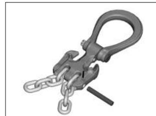
1. Place both chain links into clevis slots of fitting, insert pin fully into the two-leg clevis.
