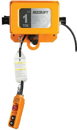
Accolift® Motorized Trolleys are rugged in design and built to be flexible right out of the box. Each trolley is adjustable for a beam flange range of 83mm to 305mm with no additional materials required. Side guide rollers are included to promote smooth trolley motion and to minimize wheel and beam flange wear.
