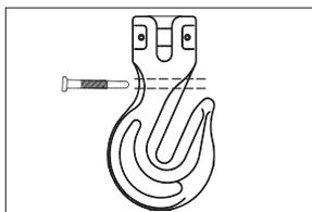
**Step 2:** Insert new S-4338 pin assembly into hook.
