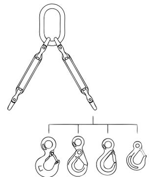
\* Ultimate load is 5 times the Working Load Limit. † L-320AN Style Hook.
