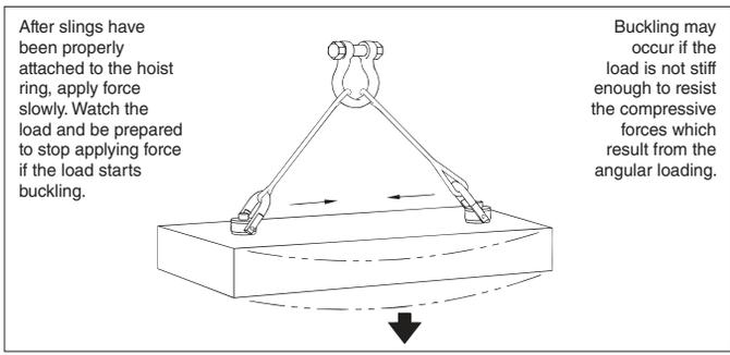
Ω Ultimate Load is 4.5 times Working Load Limit for 7000# Hoist Ring when tested in 90° orientation. All sizes are individually proof tested to 2-1/2 times the Working Load Limit. \*, †, ††, ‡ (See footnotes at bottom of Table 5).
