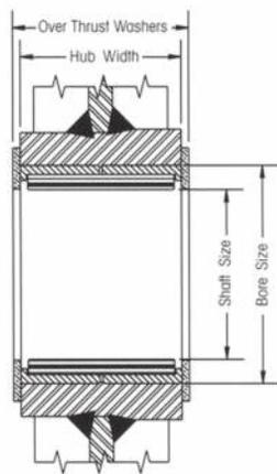
Roller Bearings without inner races are designed to operate on shafts carburized to 60 Rockwell C and grounded to +/- .0005 of shaft size.
