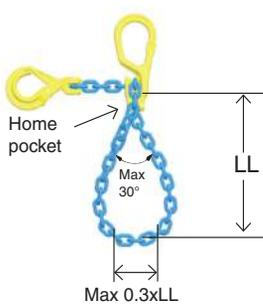
Home pocket loop shall have an internal loop top angle of max. 30°. Rule of thumb: Cross dimension of the load shall be max. 0.3 times the loop length (LL)
