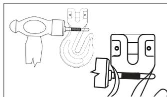
**Step 3:** Using hammer, tap lightly on latch pin head until guide bushing shoulder touches hook.
