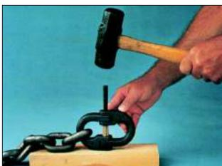
2. Drive the pin through the assembled link ends and sleeve until the end of the pin is flush with the outside of the connecting link halves.
