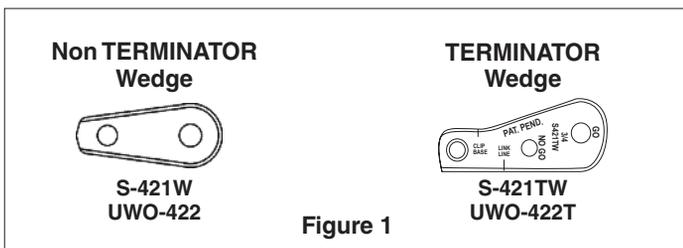
**QUIC-CHECK®** "Go" and "No-Go" features cast into wedge. The proper size wire rope is determined when the following criteria are met:
