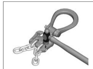
2. Place Eliminator assembly on a firm surface. Using a hammer, drive the locking pin into the two-leg clevis until it is flush with the top of the hole.
