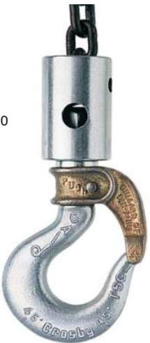
With ball-bearing swivel; attaches to chain by an alloy pin. Suitable for frequent rotation under load. Hook sizes: 4, 5, and 7.
