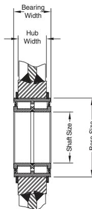
Cylindrical Roller Bearings with snap ring grooves are complete units with outer and inner rings, rib-guided cylindrical rollers, and sealing rings. They can support axial forces in both directions, as well as radial forces. They have high dynamic and static load ratings.
