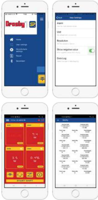
The app records total loads, weights and lifts. This feature is useful when a particular measurement(s) is required for later referral. Added to this is the option to set the threshold and measure productivity for each load cell and the device it's rigged to, a crane, for instance, for analysis to see shortfalls and improve performance.
