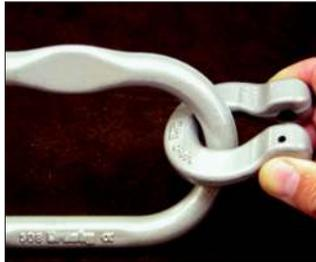
2. Rotate Coupler Link so that clevis fitting is to the outside of Master Link and attach to chain sling.
