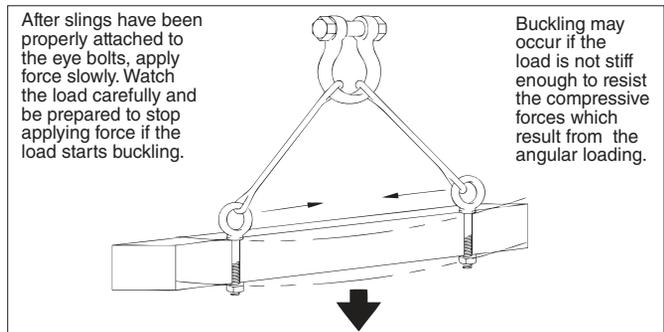
**Machinery Eye Bolt - Installation for In-Line & Angular Loading**
