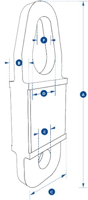
The Crosby Straightpoint Towcell® is a 25kN wireless loadcell, specifically engineered for the emergency services, salvage, and 4x4 industries. The Towcell allows for increased safety and the avoidance of costly overloads by providing real-time monitoring of tensile towing forces during recovery, clearance and salvage efforts.
